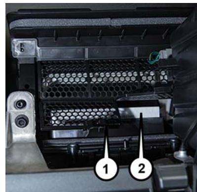
Air Filter Access Door Open
