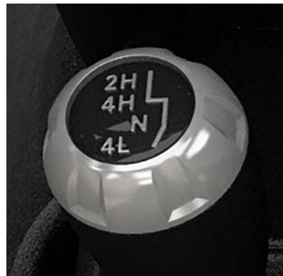
Four-Wheel Drive Shift Pattern
