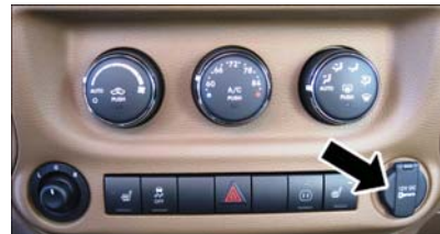
Power Outlet — Front
