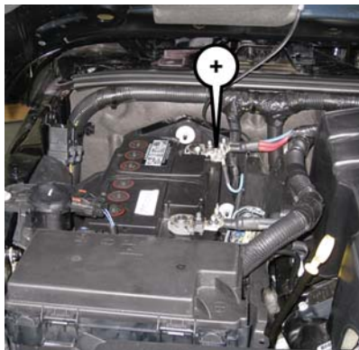
Positive Battery Post
