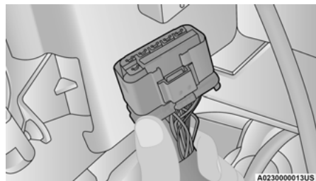
Pull Wiring Harness To Separate
