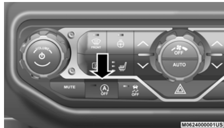
Stop/Start OFF Switch
