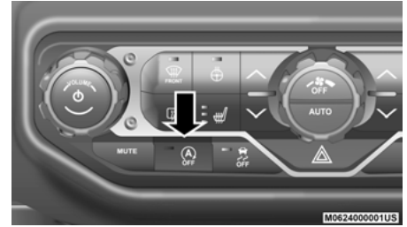
Stop/Start OFF Switch
